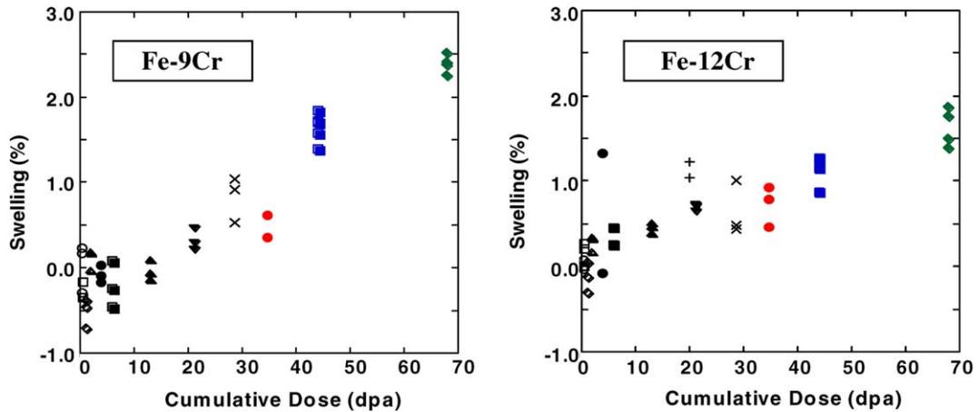
Fig. 2. Swelling of two simple model bcc Fe–Cr alloys in FFTF-MOTA at  $\sim 400$  °C, as observed in the current experiment, showing some early densification but no apparent dependence of swelling on dpa rate.
